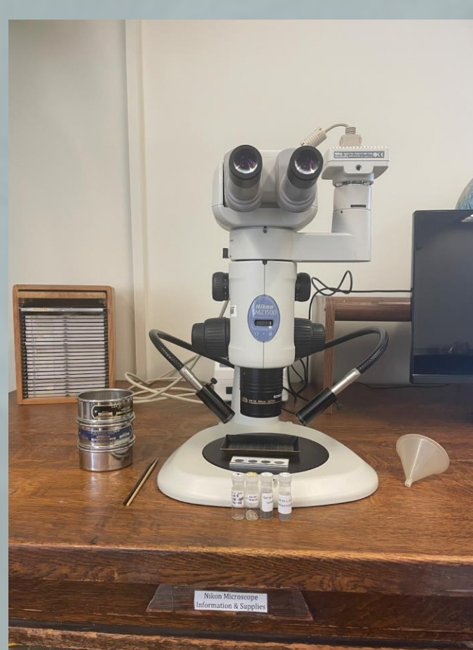
Figure 3. Nikon SMZ-U Stereomicroscope and >250 \mu m and >125 \mu m sieves used to identify foraminifera
