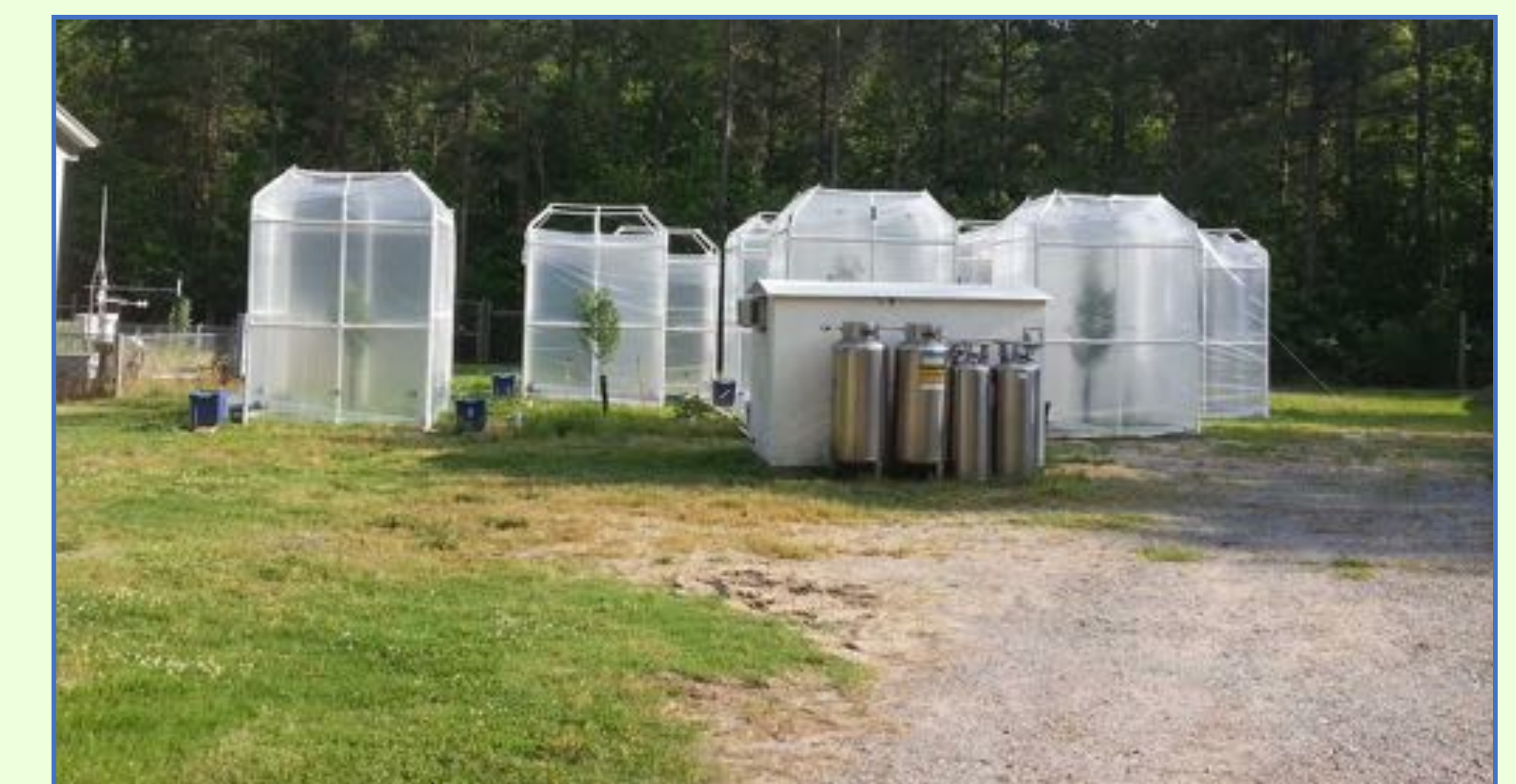
Figure above: experimental open-top CO 2 chambers with G. biloba .
