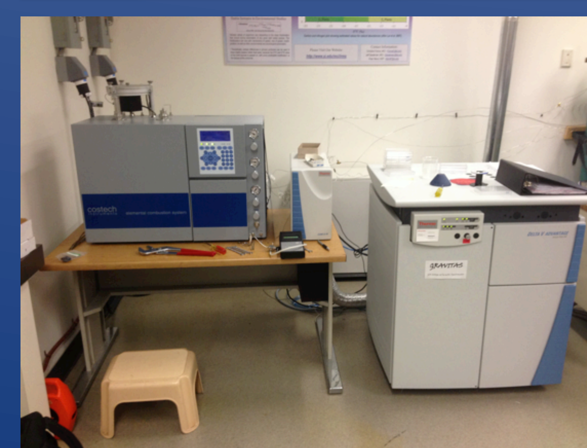
(Left): Elemental Analyzer and Mass Spectrometer used for stable isotope analysis
